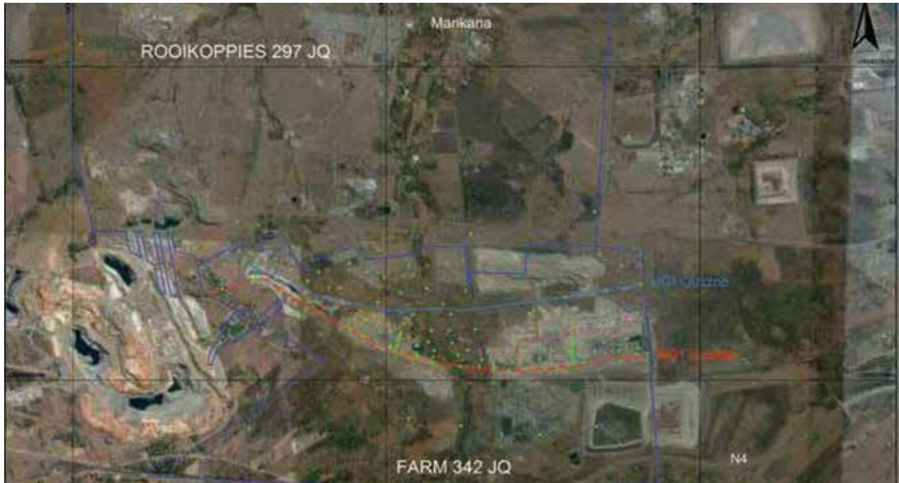
Figure 2: Image of the Tharisa Mine plan showing borehole locations and outcrop positions of UG1 and MG1 chromitite layers
