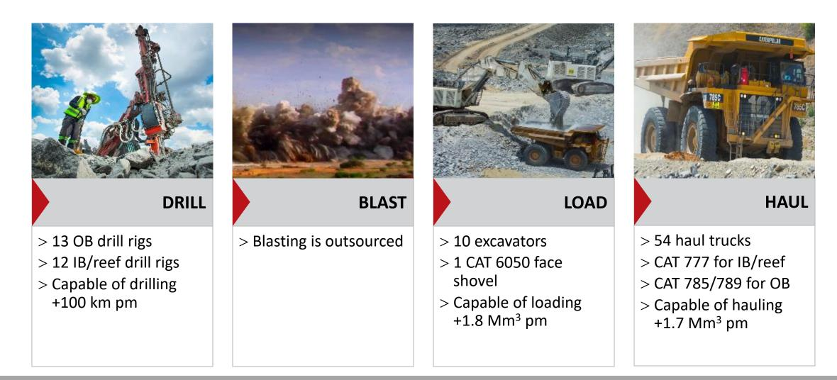
Current fleet capable of mining the 5.6 Mtpa of reef and more than the life of mine average stripping ratio to meet Vision 2020 targets
